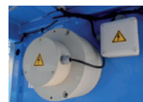
Overspeed parachute with auto-recovery system
