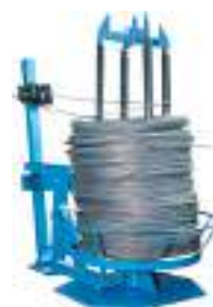
Decoiler for uncoiled wire rod
