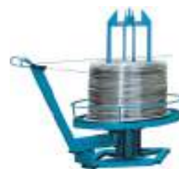
Decoiler for coiled wire rod
