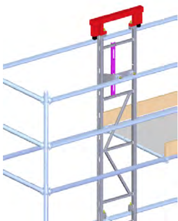
CORRECT / INCORRECT POSITION OF UPPER ENDTRACK CAM - STANDARD
