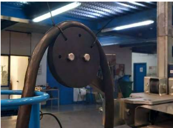
Fitting the cable on hanging bracket
