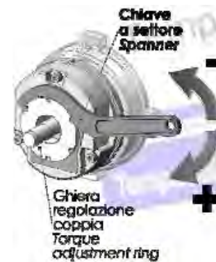
ADJUSTING BRAKE AIRGAP AND TORQUE (SINGLE PHASE MOTOR)
